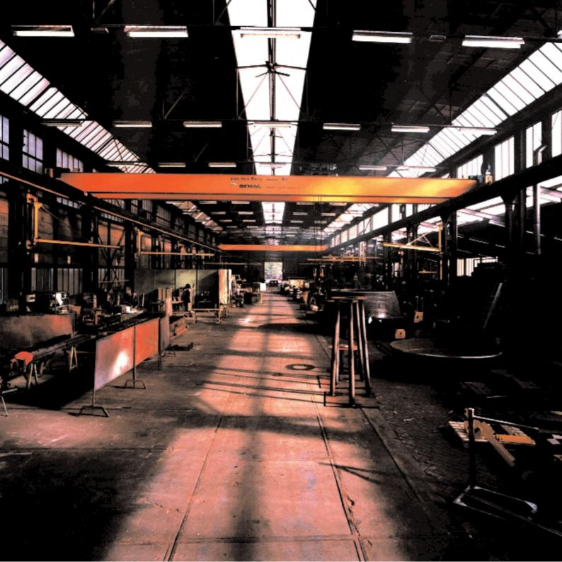
In Belgium, GreenLight Partner Beerse Metaalwerken nv replaced the standard high pressure mercury lamps of their workshop with 26 mm diameter fluorescent lamps. They also installed a control system to dim the lamps' output in response to daylight availability. In their offices, they replaced the 38 mm diameter fluorescent lamps with 26 mm diameter lamps. All new lamps are geared with electronic ballasts.
